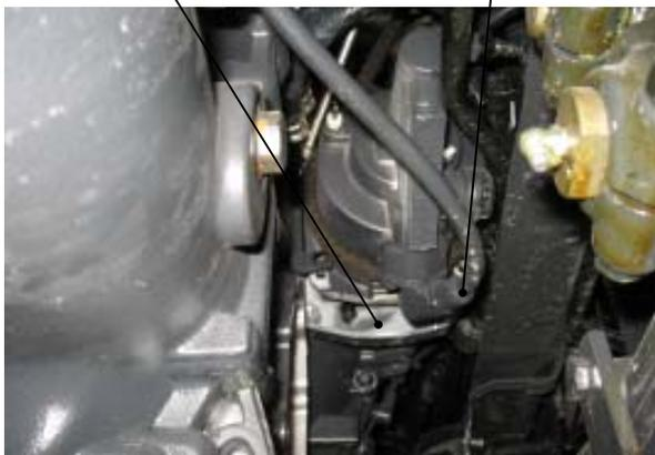
Unscrew the screws completely from the clutch cylinder and move it slightly (E), with great care, **DO NOT REMOVE IT COMPLETELY**. Turn the cylinder slightly, moving the obstruction of the tube (F), slowly
