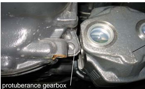
In case you use one of our pumps (pictures are showing our HDS and NPH... THIN ISO SHORT types) please take care that the gearbox tab (due to casting tolerances) does not interfere against the pump itself, jeopardizing in this case its correcting mounting, use and lifetime. If needed, please clear this interference by means of the most appropriate tools.
