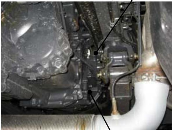
Preliminary operation: drain the oil from the gearbox. The picture shows the PTO attachment flange (A), and the clutch cylinder to be moved (B).
