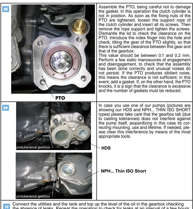
the absence of leaks. Repeat the operation to check for leaks at an interval of a few hours.
